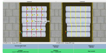
The image shows a complete 3D stereo vision simulation generated from the 3D model. This reduces deployment cost of Scorpion 3D Stinger systems.
